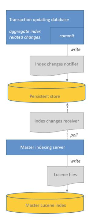
Figure 405: Indexer architecture in a single-server environment
