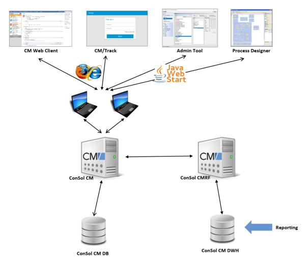
Figure 381: ConSol CM - System architecture with DWH and CMRF (2 servers)
