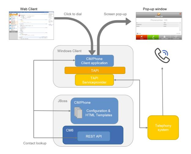
Figure 718: ConSol CM/Phone - Basic principle
