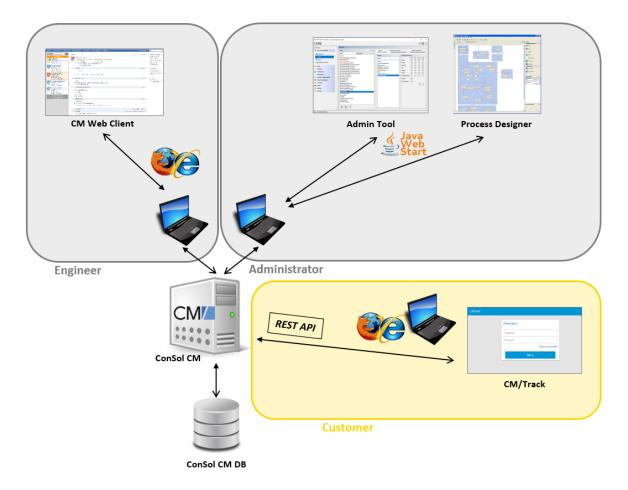
Figure 673: ConSol CM system architecture with CM/Track
