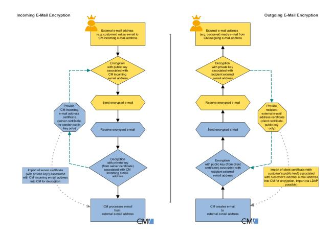
Figure 450: Basic principle of ConSol CM email encryption
