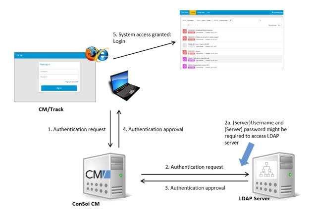
Figure 677: ConSol CM - LDAP authentication process for CM/Track
