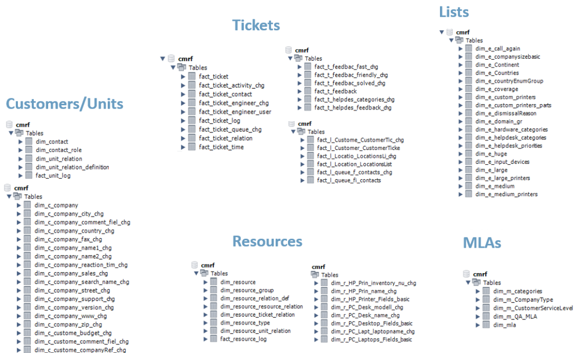
Figure 4: Table naming conventions: Example tables from the DWH database of the documentation scenario
