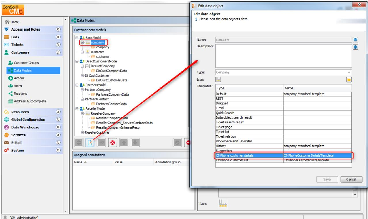
Fig. 8: ConSol CM Admin Tool - Assignment of CM.Phone Templates for Customer Data to Customer Groups
