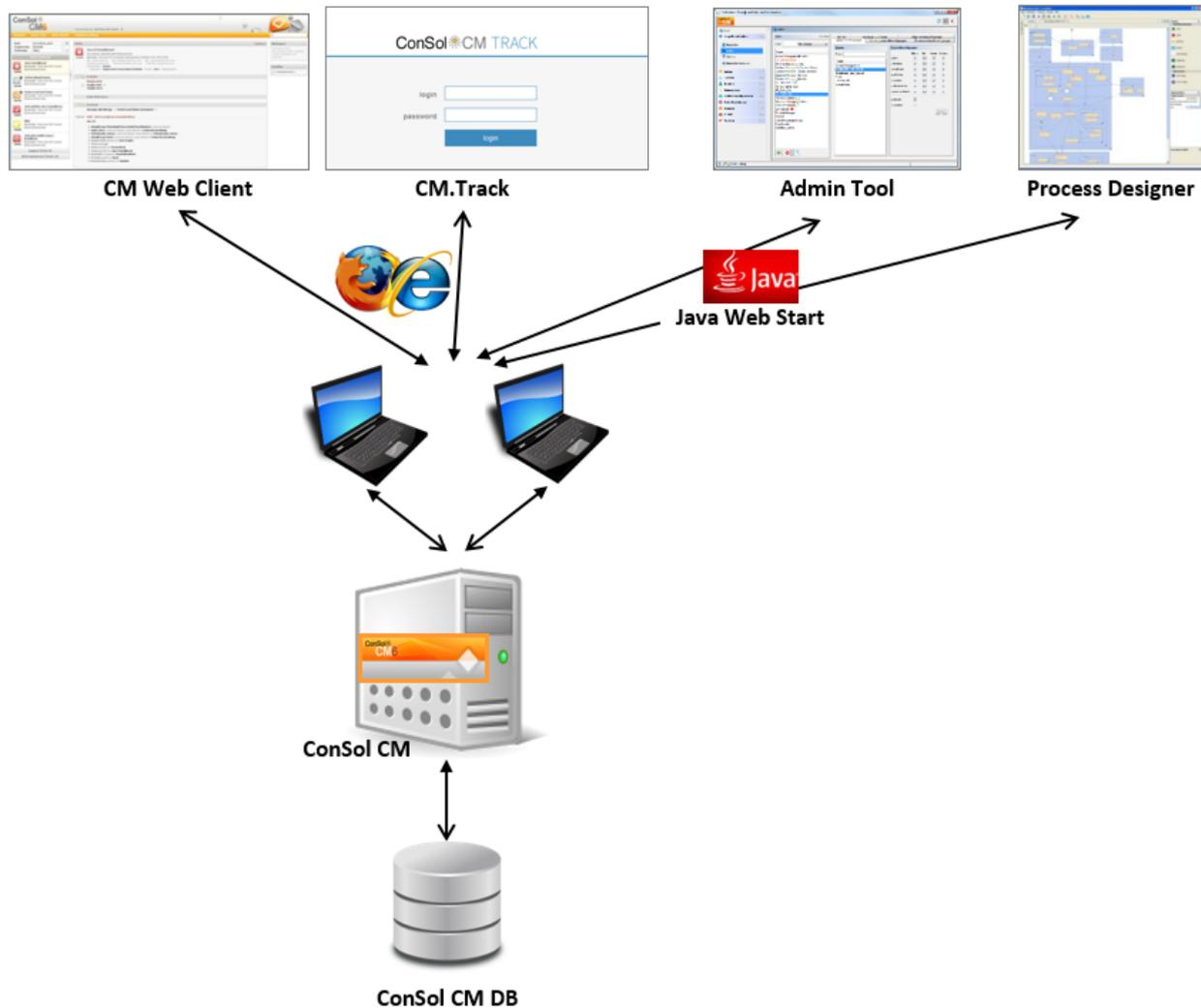
Fig. 1: ConSol CM - Basic System Architecture
