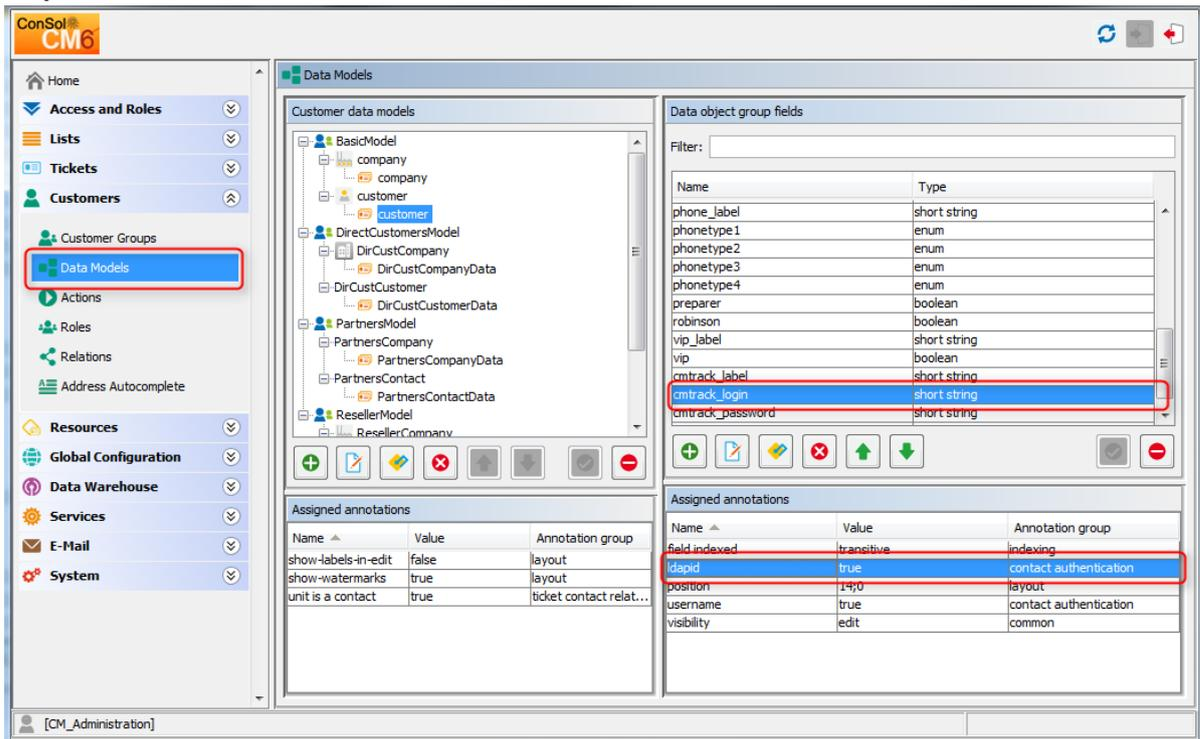
Fig. 1: ConSol CM Admin Tool - Data Object Group Field for LDAP Authentication of CM.Track users
