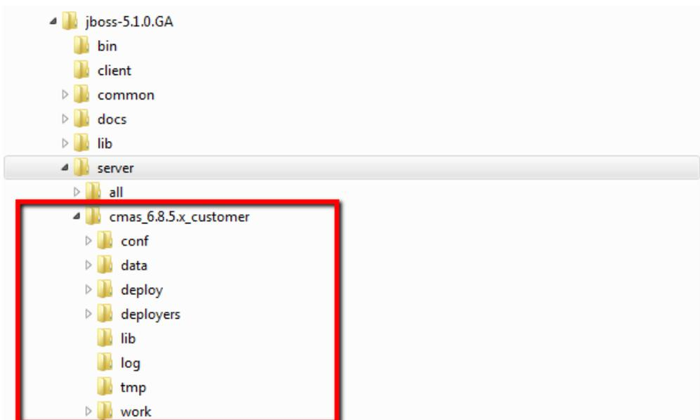
Fig. 5: ConSol CM - File Structure in a JBoss 5 Application Server
