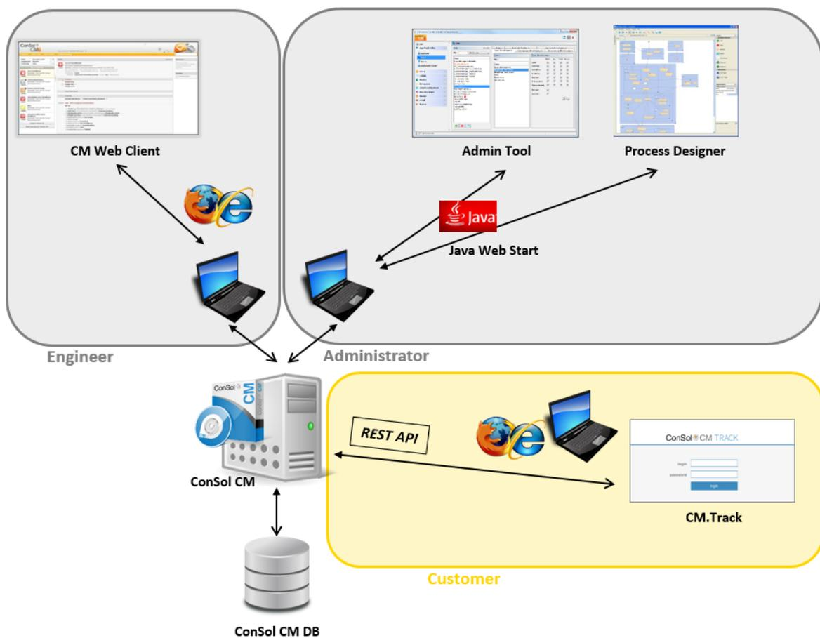
Fig. 1: ConSol CM System Architecture with CM.Track
