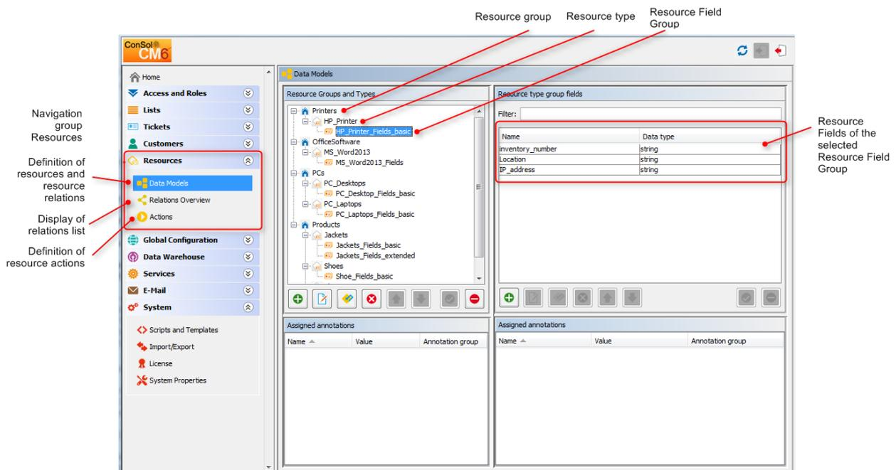
Fig. 1: ConSol CM Admin Tool - Main Elements for the Configuration of CM.Resource Pool
