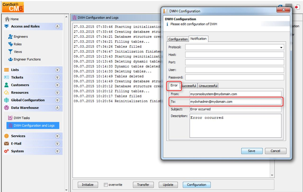
Fig. 2: ConSol CM Admin Tool - Notification Address for DWH Errors
