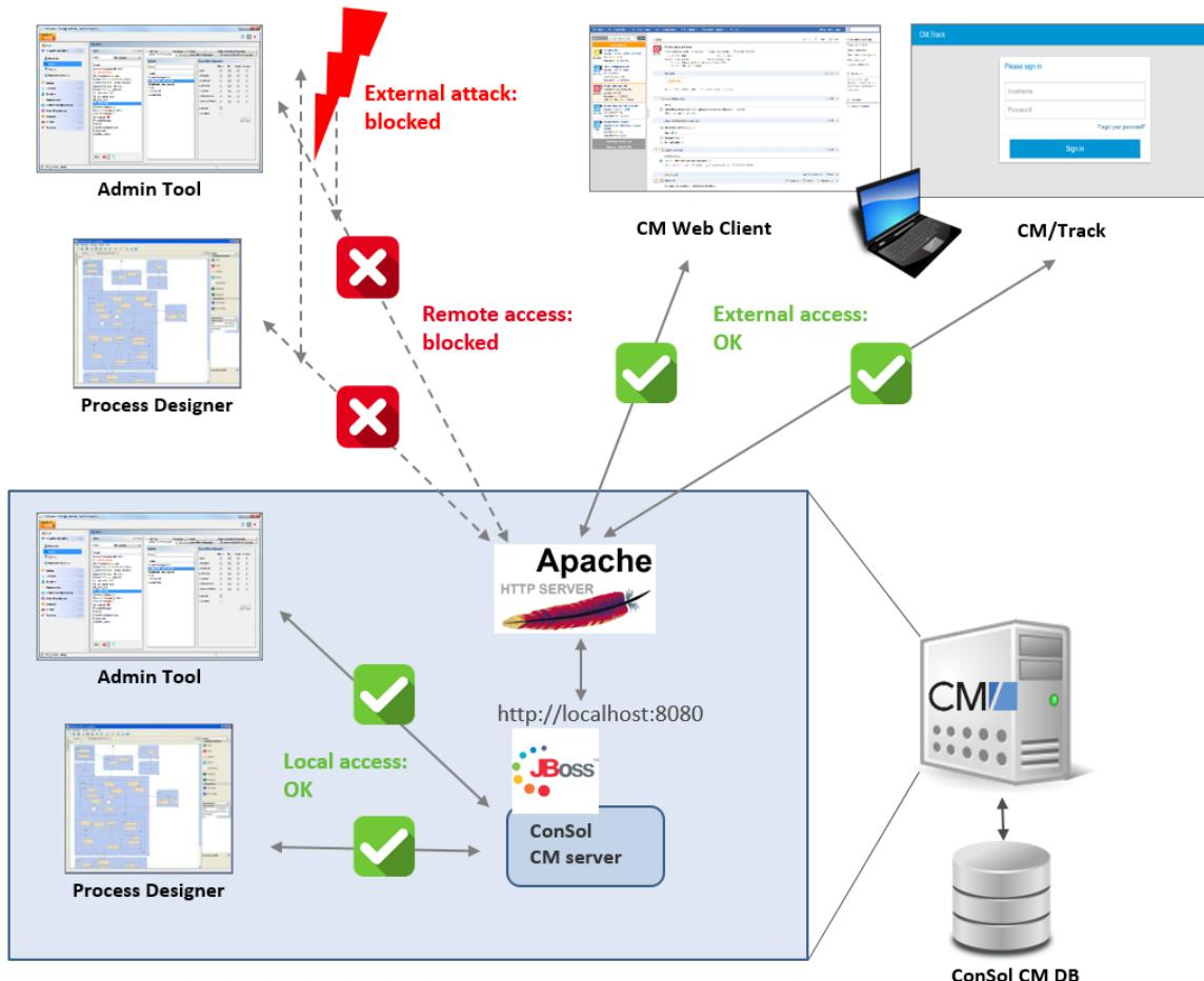
Figure 11: Operating ConSol CM behind a proxy server (here Apache HTTP server)
