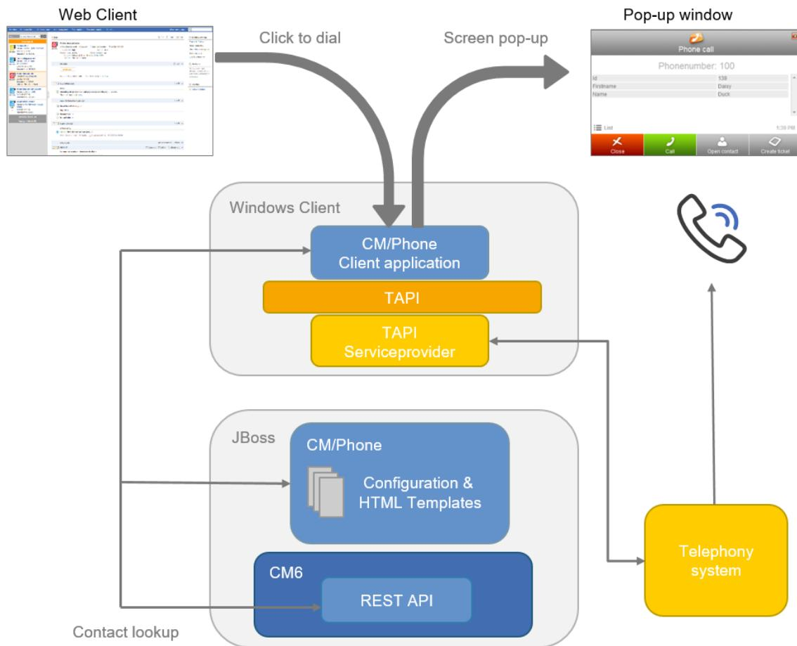
Figure 32: *ConSol CM/Phone - Basic principle*
