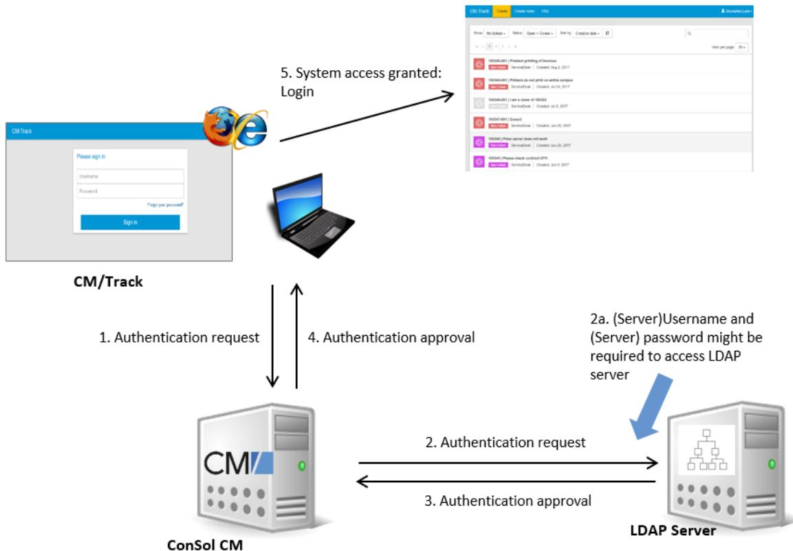
Figure 31: ConSol CM - LDAP authentication process for CM/Track
