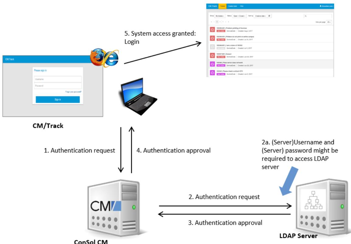
Figure 29: ConSol CM - LDAP authentication process for CM/Track
