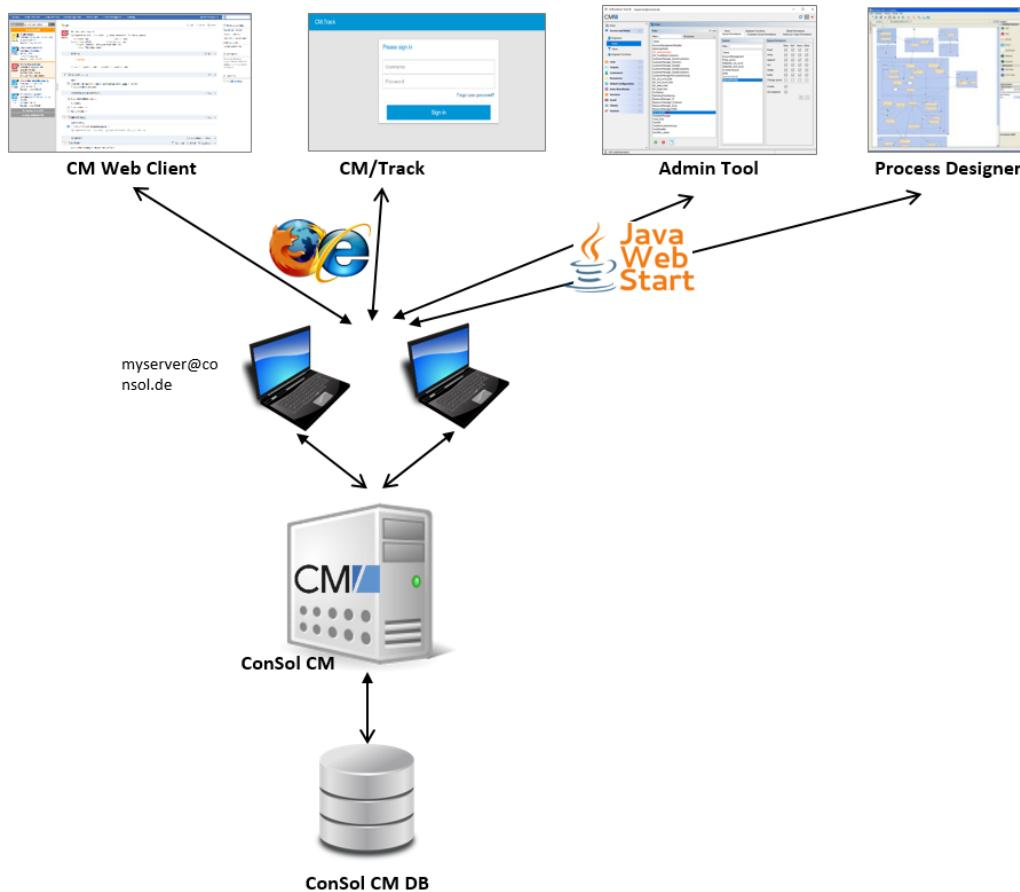
Figure 3: *ConSol CM - Basic system architecture*
