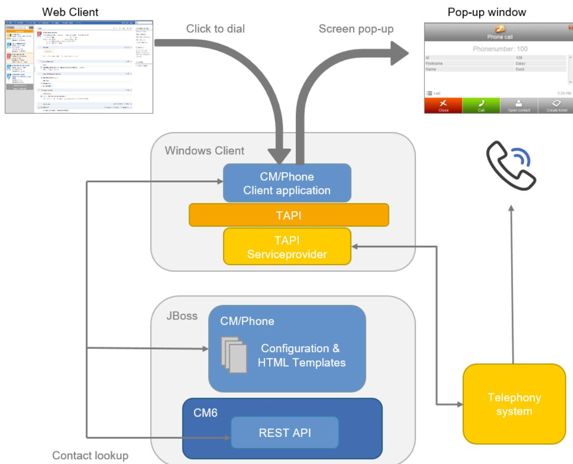
Figure 29: *ConSol CM/Phone - Basic principle*
