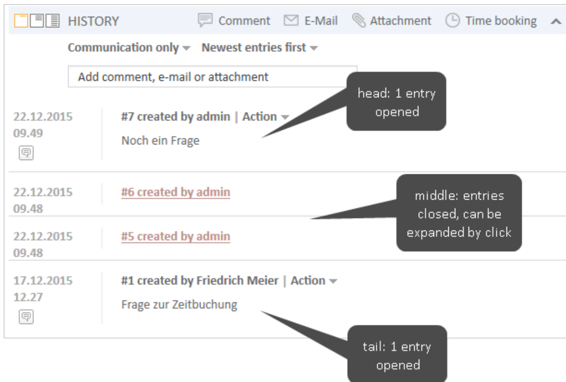
Figure 142: ConSol CM Web Client - headHistoryElementsCount and tailHistoryElementsCount set to 1
