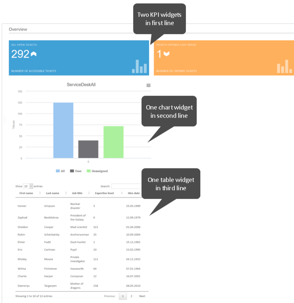
Figure 201: ConSol CM Web Client - Dashboard with four widgets of different types
